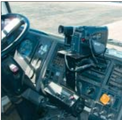
A simple off-the-shelf, dash-mounted video camera sits on a mounting bracket, both of which were purchased from a police equipment company.
